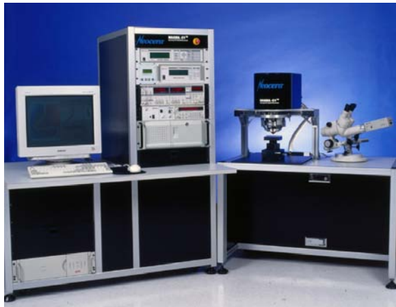
Figure 1 Photograph of the commercial scanning SQUID microscope, MAGMA-C1, with electronics rack and probe station.
