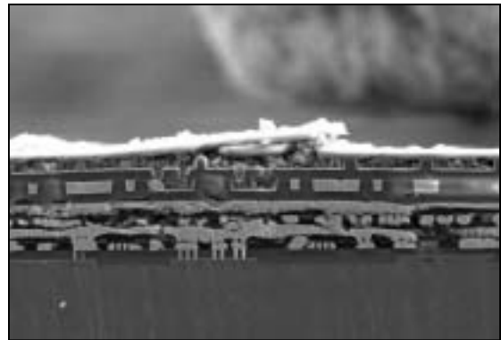
Figure 11: SEM cross-sectional image of shorting site identified in fig.'s 7-10.
