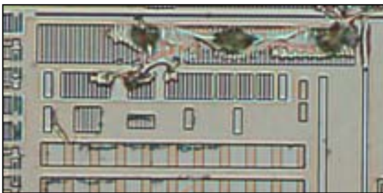
Figure 2: Optical image of typical NFET overload site at silicon level.
