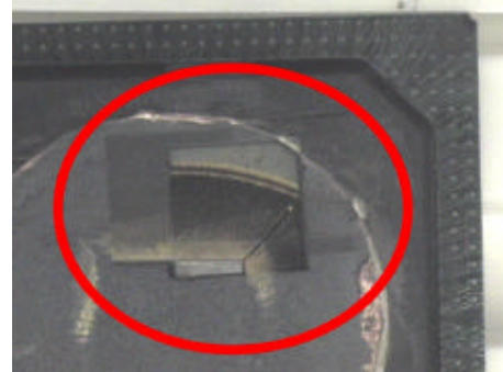
Figure 11 Optical image of the device where mold compound was partially removed by a laser decapsulation tool
