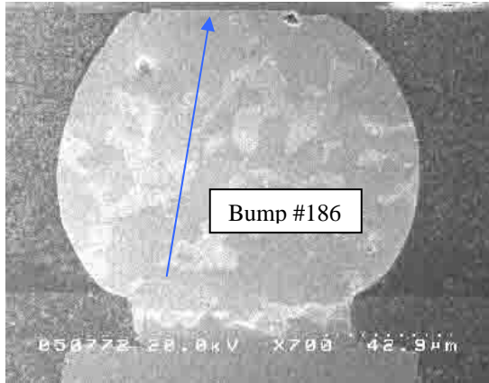
Figure 19 SEM image of solder bump 186 of pin F4. The crack is indicated by an arrow
