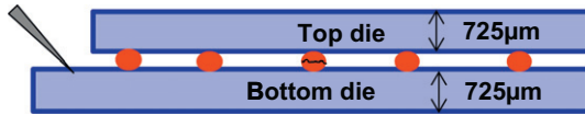
Fig. 3. Side view of the double stacked die connected using microbumps in a daisy chain structure with a cracked bump showing open on electrical test measurement.
